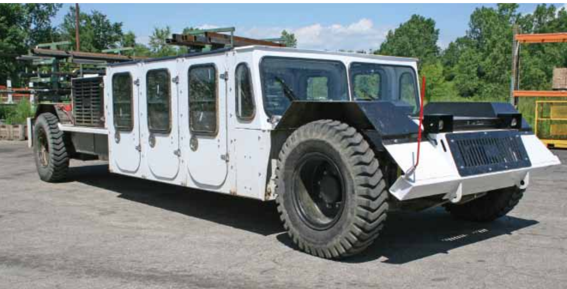
The Getman GT12 prototype features diesel power, four-wheel-drive, and a very tight turning radius. Baril's DCC paint replaces the galvanized components that Getman's line of TerraPro personnel carriers utilized (Chad Elmore photo).
